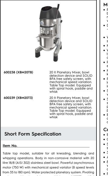
and removable wire safety screen. Water proof (IP55) and flat touch button control panel with 60 min. timer. A safety device will automatically stop the machine when the bowl is lowered. Removable and dismantled solid safety screen - made of a bisphenol-A free (BPA) copolyester. Bowl detction device allows the mixer to switch on only when the bowl and the safety screen are properly installed and positioned together. Adjustable feet for stability.
