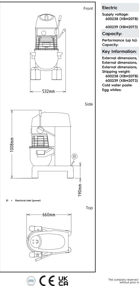
Capacity:6 kg/Cycle<br/>20 litresPerformance (up to):6 kg/Cycle<br/>20 litresCapacity:20 litresKey Information:521 mmExternal dimensions, Width:521 mmExternal dimensions, Depth:685 mmExternal dimensions, Height:1010 mmShipping weight:95 kg600238 (XBM20TB)95 kg600239 (XBM20T3)94 kgCold water paste:6 kg with Spiral hook
